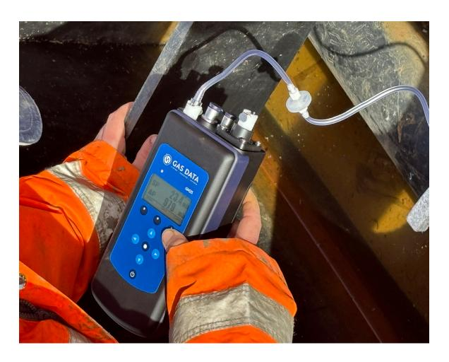
Gas Data portable gas analysers are designed for on site analysis in demanding biogas, landfill, and site investigation conditions where accurate measurements are essential. The GM25 range of gas analysers are highly accurate and reliable whilst being certified for use in potentially explosive EX Zone 1 atmospheres.
