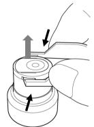
4 Place the pellet and LED on a clean surface. Separate the pellet removal tool from the VOC sensor.
